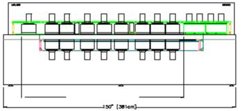
A nine-zone configuration within the reflow oven ensures the tight gas flow circulation management needed to maintain a consistent lead-free profile.
