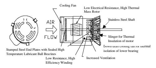
A high-efficiency ball bearing motor designed for a maximum operating temperature of 450°C helps maintain the very low **D**T required for lead-free reflow.
