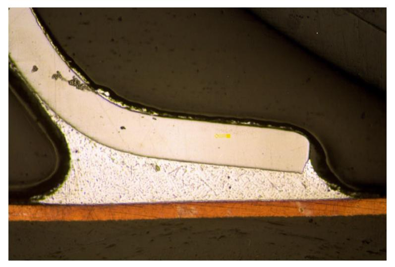
Reduced Toe and Heel Wetting in Air Acceptable Joint
